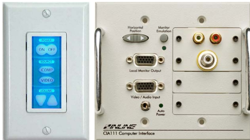
Figure 18: Control Panel and Interface Panel
