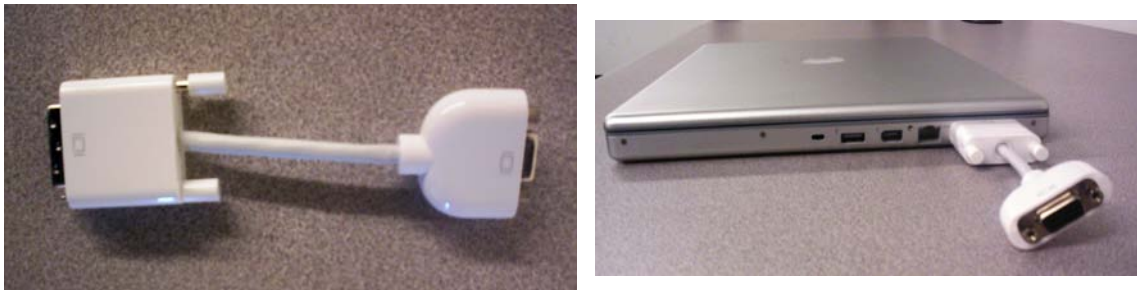
Figure 12: Apple DVI to VGA Display Adapter cable for a Mac laptop and an example of a VGA adapter cable connected to a Mac laptop
